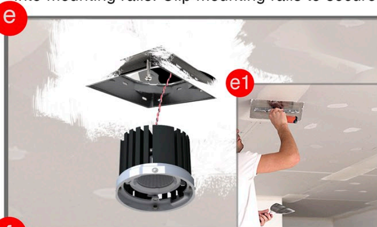
Step A- Anchor mounting rails into joists with screws. Slide Bracket Pan with butterfly brackets into mounting rails. Clip mounting rails to secure.
