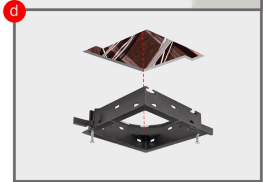
Step C- Paint over ceiling before installation. Step D- Slide receiver into ceiling.
