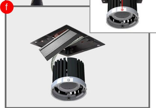
Step E- Tighten screws to clamp receiver to ceiling. Finalize electrical wiring/connections. Step F- Slide light assembly into receiver. Ball plungers(4) on light assembly clicks into 4 slots on receiver (see detail above)
