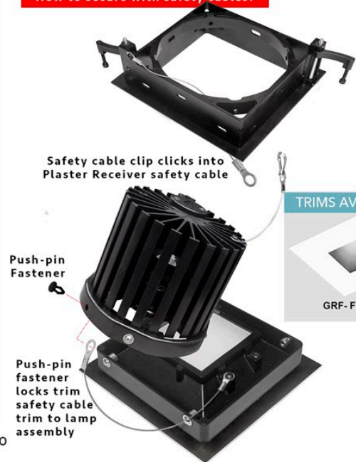
Step E- Tighten screws to clamp receiver to ceiling. Finalize electrical wiring/connections. Step F- Slide light assembly into receiver. Ball plungers(4) on light assembly clicks into 4 slots on receiver (see detail above)
