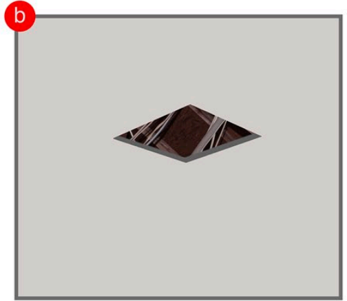
Step B- Cutout opening for light install
