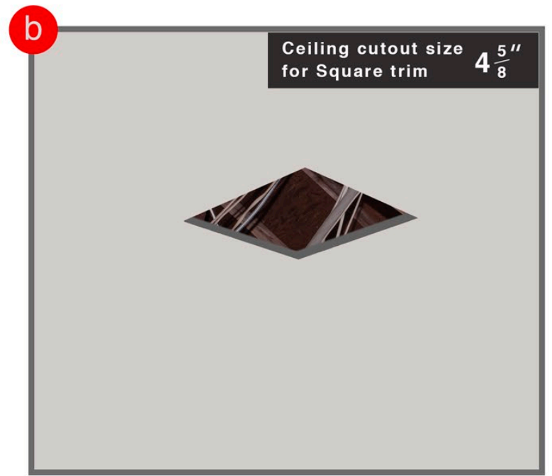
Step B- Cutout opening for light install. (Notches in square cutout are optional.)
