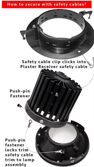
Step 4c- Slide driver enclosure with light fixture into receiver. Enclosure rests on GWB. Step 4d- Lock light fixture into receiver.
