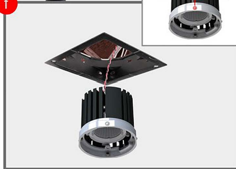
Step E- Tighten screws to clamp receiver to ceiling. Finalize electrical wiring/connections.
