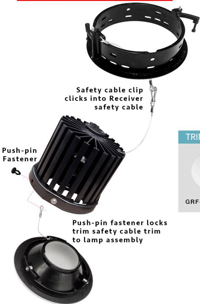
Step E- Finalize electrical wiring/connections. Then slide light assembly into receiver. Step F- Ball plungers(4) on light assembly clicks into 4 slots on receiver.
