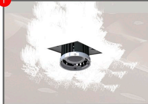
Step E- Plaster receiver flange. Finish Electrical. Step E1- Apply tape & joint compound Step F- Slide light assembly into receiver. Finish plastering GWB.
