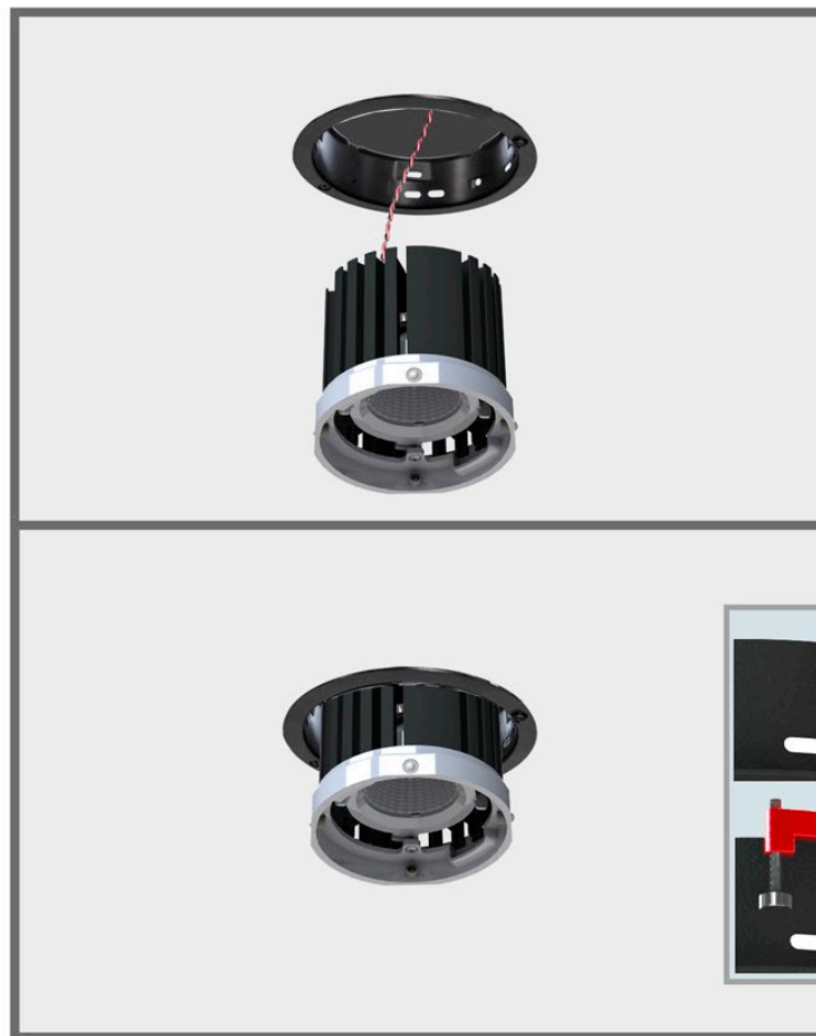
Step E- Finalize electrical wiring/connections. Then slide light assembly into receiver. Step F- Ball plungers(4) on light assembly clicks into 4 slots on receiver.
