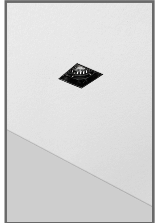
G After plaster ceiling has dried, paint over the plaster ceiling.
