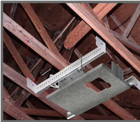
A Anchor mounting rails into joists with screws. Slide Bracket Pan with butterfly brackets into mounting rails. Clip mounting rails to secure.
