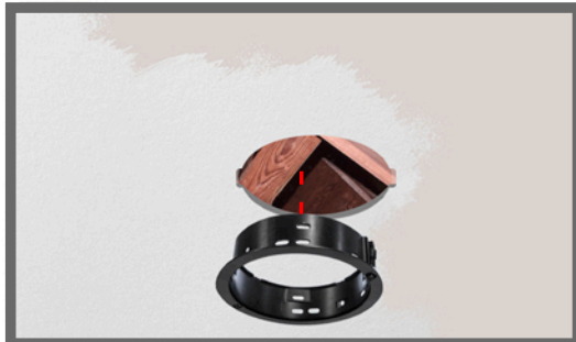
C Slide Flange receiver into opening.
