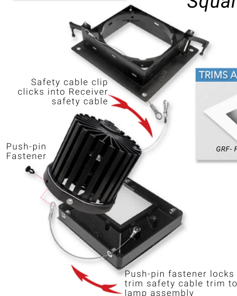
H Make sure trim ball plungers clicks into receiver to secure.
